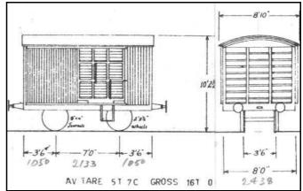
These closed 4 wheel wagons had hand actuated brakes, here is a drawing used to make the model.
